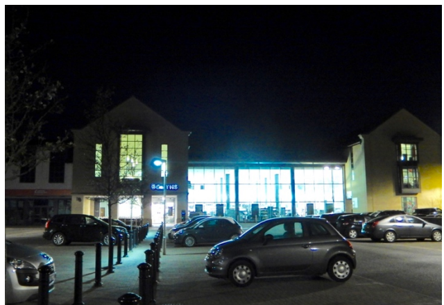
Here light spill at eye level is intentional to enhance the prominence of the store and to increase the comfort of car park users.
